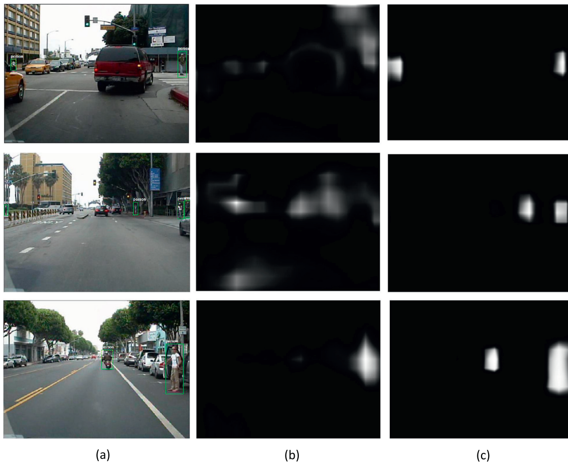
Fig. 5. Visualization of “person” channel of different FCN models outputs. (a) shows three images from Caltech pedestrian dataset. The green bounding boxes are ground truth of pedestrians. (b) shows the visualization of FCN-32s model’s “person” channel. (c) shows the visualization of fine-tuned FCN-32s model’s “person” channel.
